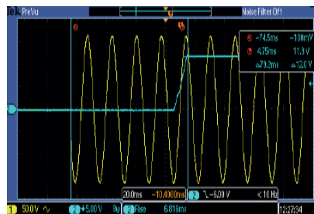
Typical Input Start-Up and Output Rise Characteristic V_{in}=V_{in\ nom} ; Full Load (-Vout)
